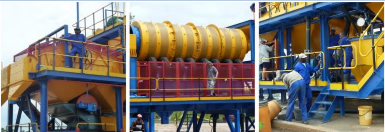
Fig. 7: Diamond Plant - 150t per hour modular treatment plant
