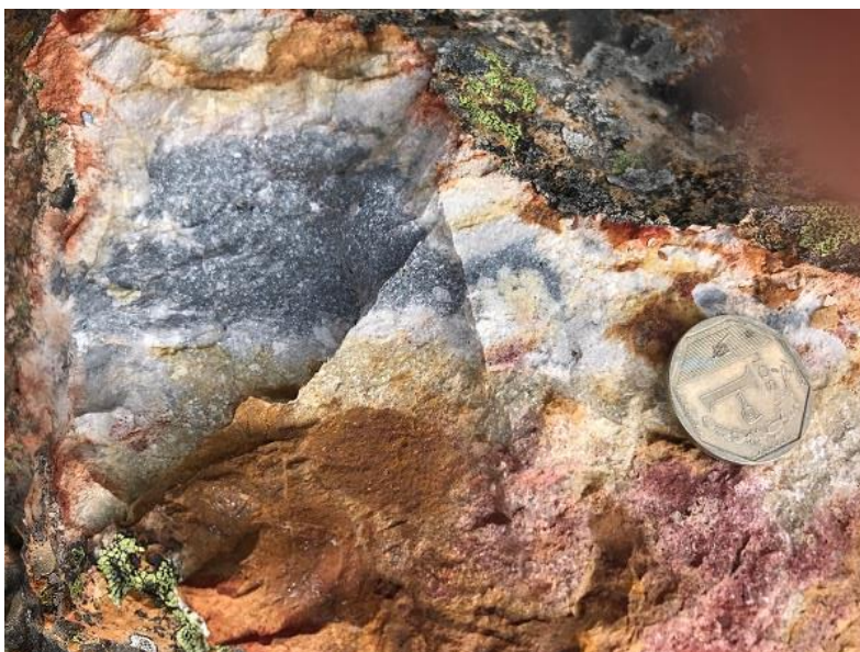
Figure 12-4: Sample 60110, very fine dark sulphides in siliceous breccia
