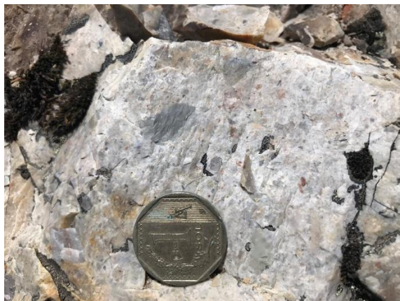
Figure 12-6: Sample 60112, siliceous, vuggy breccia with fragments of Chimu quartzite
