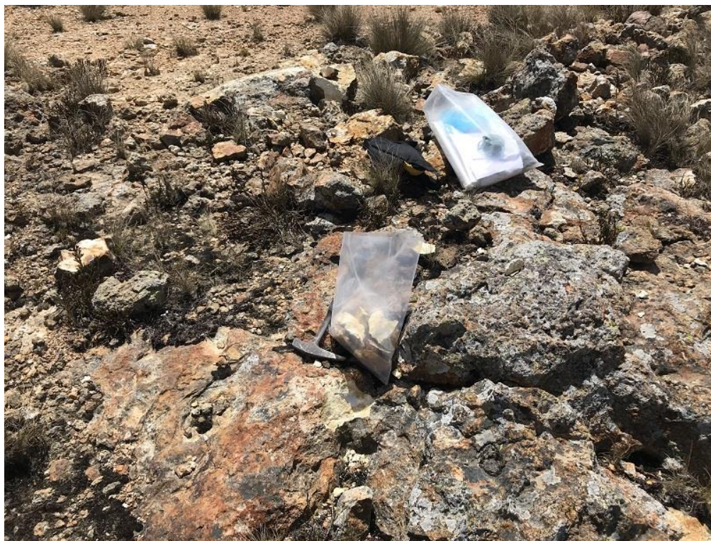
Figure 12-3: Sample 60109, 0.662 g/t Au in siliceous andesite breccia
