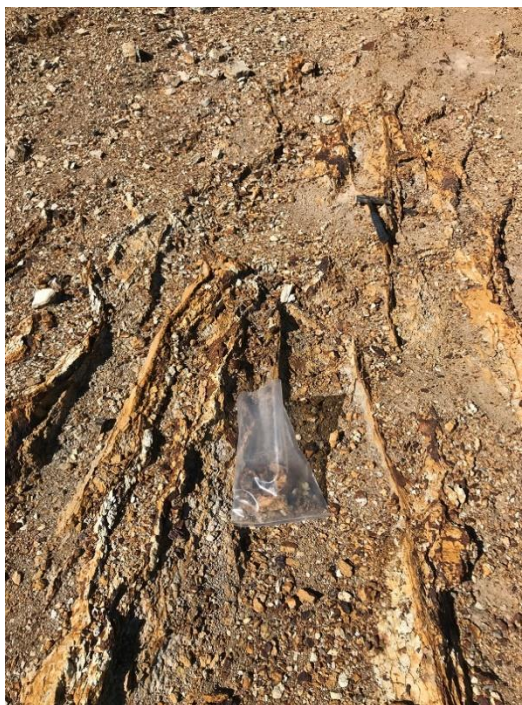
Figure 12-8: Sample 60116, Oxidized siliceous veins in altered andesitic volcanics
