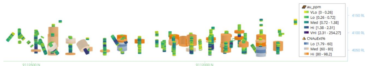
Figure 13-4: Sample Au extraction performance looking East against drilling Au grades
