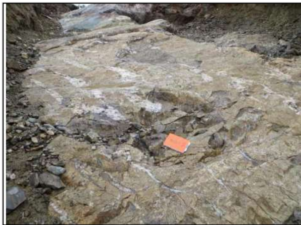
Figure 7-8: Sheeted, Shallow Southwest-Dipping Quartz Tourmaline Pyrite Vein Array (Set 1), Marathon Deposit
