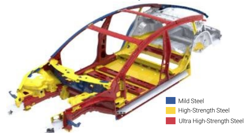
Tesla Model 3 Body Structure
