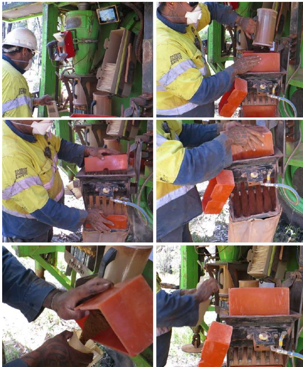
Figure 7-4: Sample Catching and Riffle Splitting Practices (SLR, 2021)
