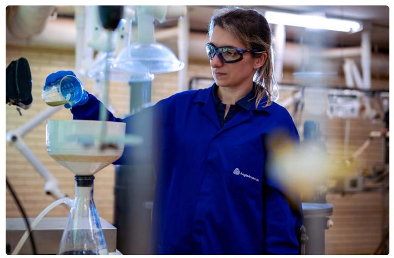
Process engineer Naiara Nascimento working with a pregnant leach solution enriched with soluble nickel, derived from comprehensive tests conducted in the leaching pilot plant at our Barro Alto operation in Brazil.
