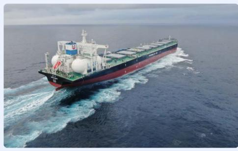
The Ubuntu Equality is the second of 10 LNG dual-fuelled Capesize+ vessels in our chartered fleet. Our LNG dual-fuelled Capesize+ vessels are estimated to deliver a 35% reduction in CO<sub>2</sub> emissions compared with similar vessels fuelled by conventional marine oil fuel.
